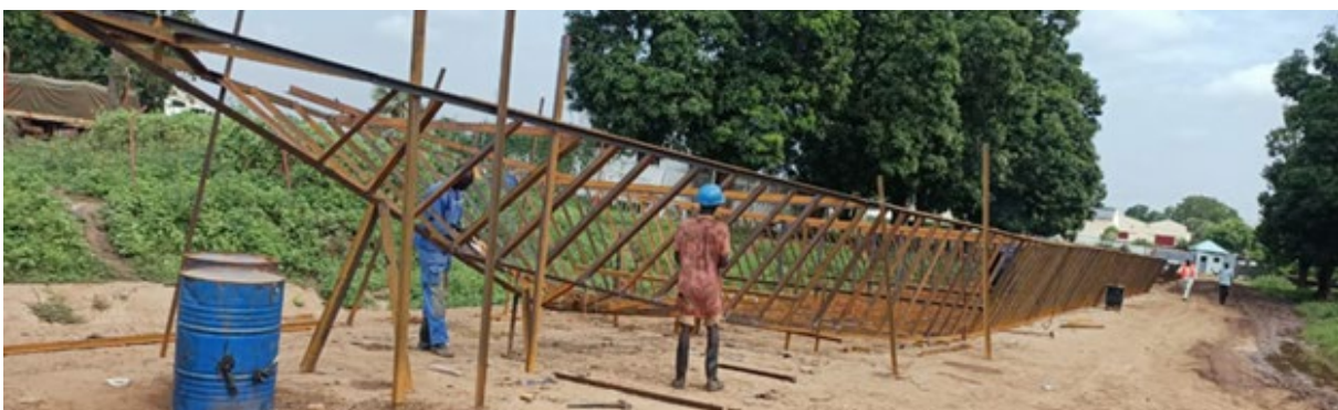
Artisans at Juba Port fabricating a boat (with length of about 40 m) to be used on River Nile. Sensitization on waterways safety and harmonization of legal and regulatory framework for inland water ways is critical. Aspects of safety should be considered right from the time of constructing the floating crafts to minimize risk of accidents in future that may arise as a result in design of the watercrafts.
